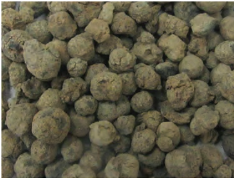
Figure 3: Sintered fly ash lightweight aggregate [15]
