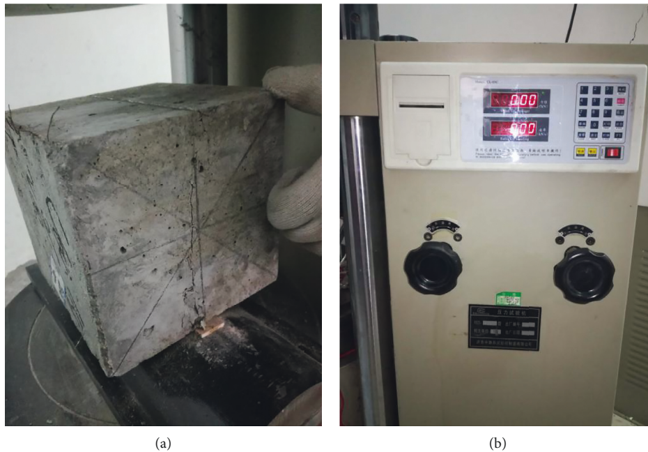
FIGURE 7: Cube splitting tensile strength testing equipment.
