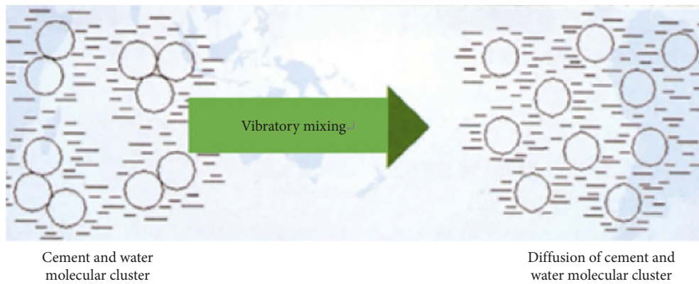
FIGURE 3: Contrast of effect between vibratory mixing and traditional mixing.
