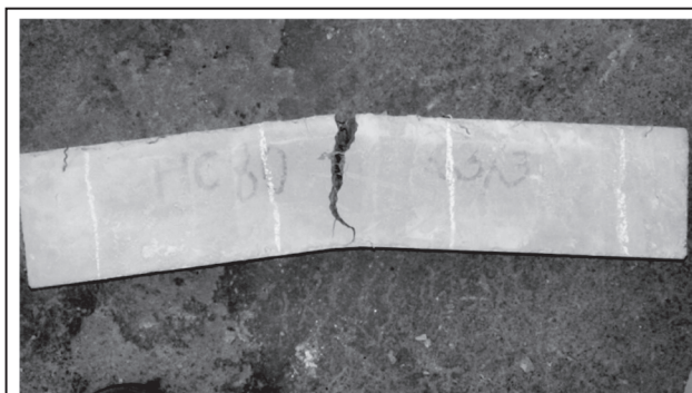
Fig. 9 Failure of sample under two point loading test
