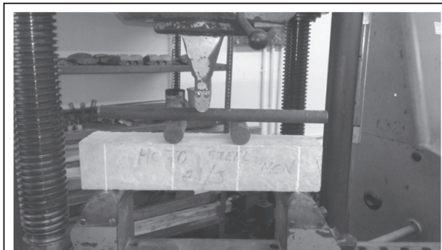
Fig. 8 Two point loading test setup in UTM
