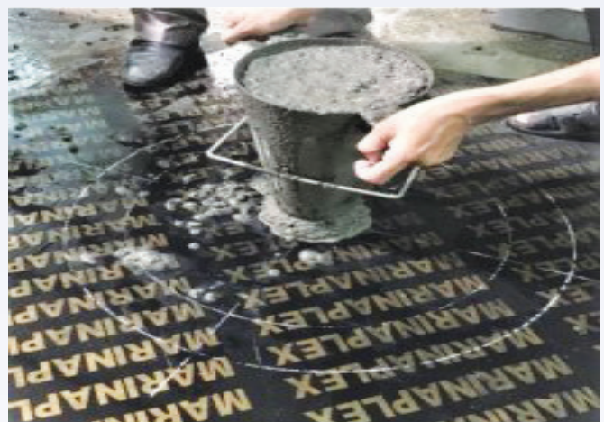
T 500 test of SCC (Time required to pass 500mm dia.)
