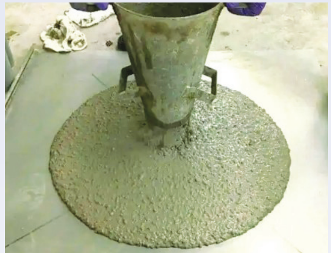
Slump flow test of SCC
