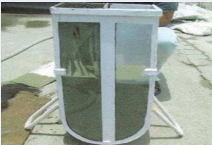
U Box test of SCC
