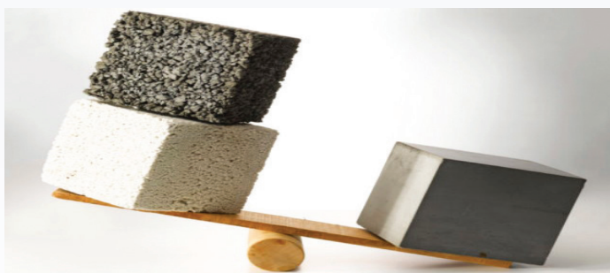
Light weight concrete
