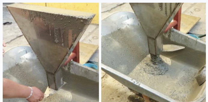
V Funnel test of SCC
