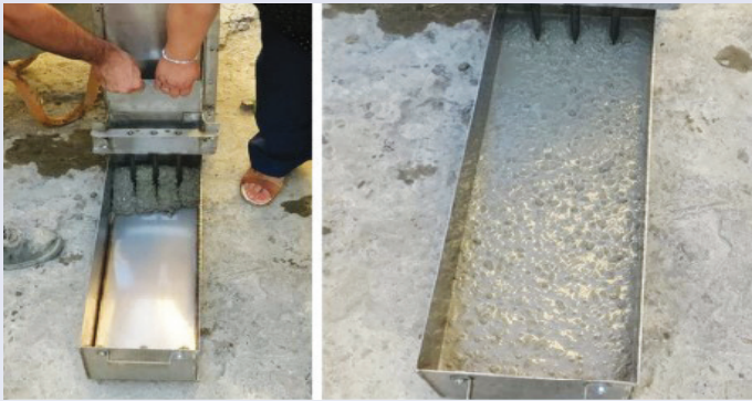
L Box test of SCC
