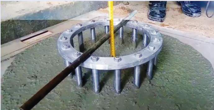
Ring test of SCC
