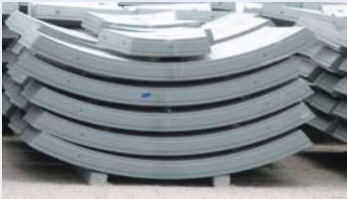
HPC – Achieving 25 MPa strength in 24 hours without steam curing (Very high early strength)
