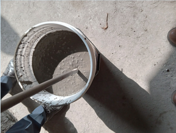
Figure 5 - The Self-Compacting Concrete after Thorough Compaction. No Segregation Observed.
