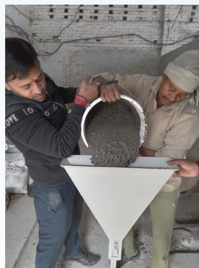
Figure 4 - The Fresh Concrete is being Poured for V-Funnel Test
