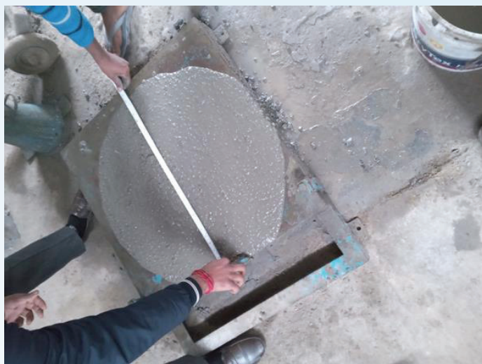
Figure 3 - The Slump- flow(650mm) of Self-Compacting Concrete after 3 hours
