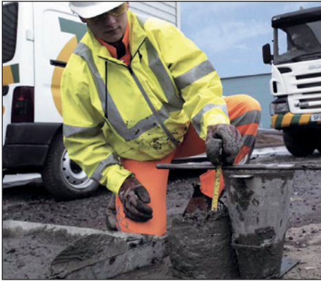
Figure A.1 Sampling from concrete stream
