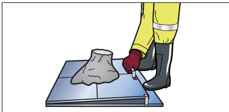
Figure B.9 Table lifting and dropping
