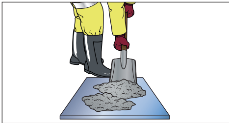
Figure B.1 Remixing sample on tray
